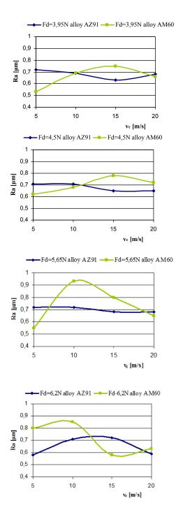
Figure 4 Ra parameter as a function of cutting speed for variable downforce material to wire
