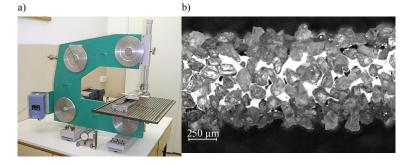
Figure 2 Research position and tool applied in examinations: a) general view of the cutting machine, b) view of the active surface of HK wire
