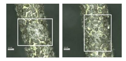
Figure 5 Local areas of fulfilled chip space on wire active surface
